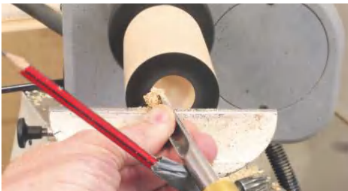
▲ Pic.15 As the hole gets deeper, you will need to close the flute off slightly as you come up the side of the hollowed area. The pencil is now telling me it's at 10 o'clock
